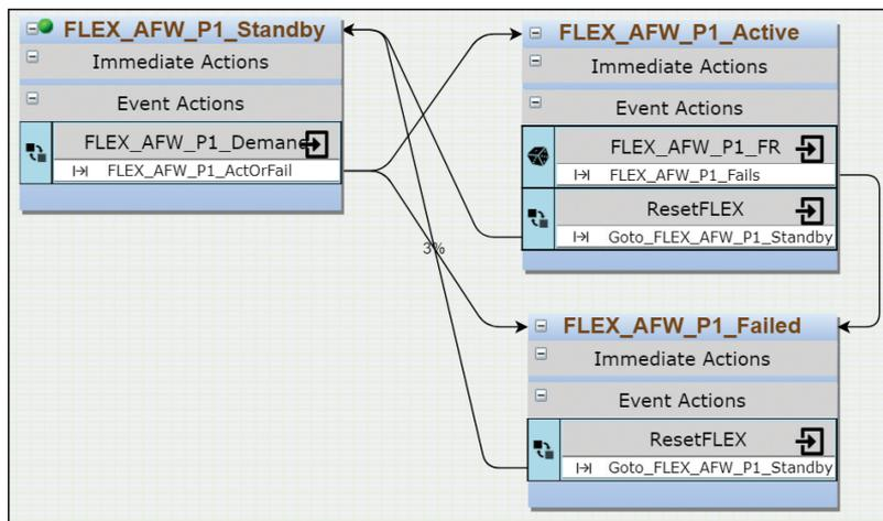
Fig. 14. Diagram of FLEX pump's operational states.
