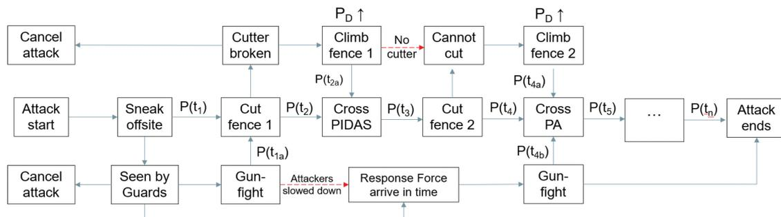
Fig. 4. Possible variations of an attack plan.
