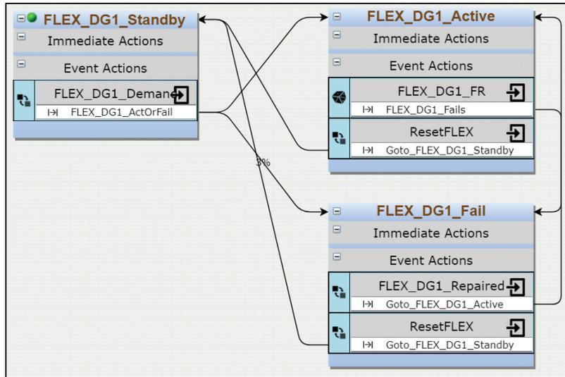
Fig. 13. Diagram of FLEX generator's operational states.
